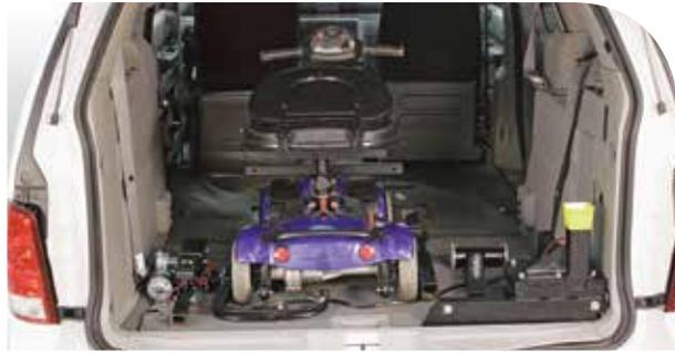
Take-apart lift disassembles when not in use if desired.
