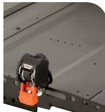
3 retractable self-tensioning securement belts with one hand operation.
